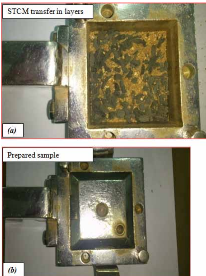
Figure 2. Typical photographs of STCM sample preparation for direct shear test
