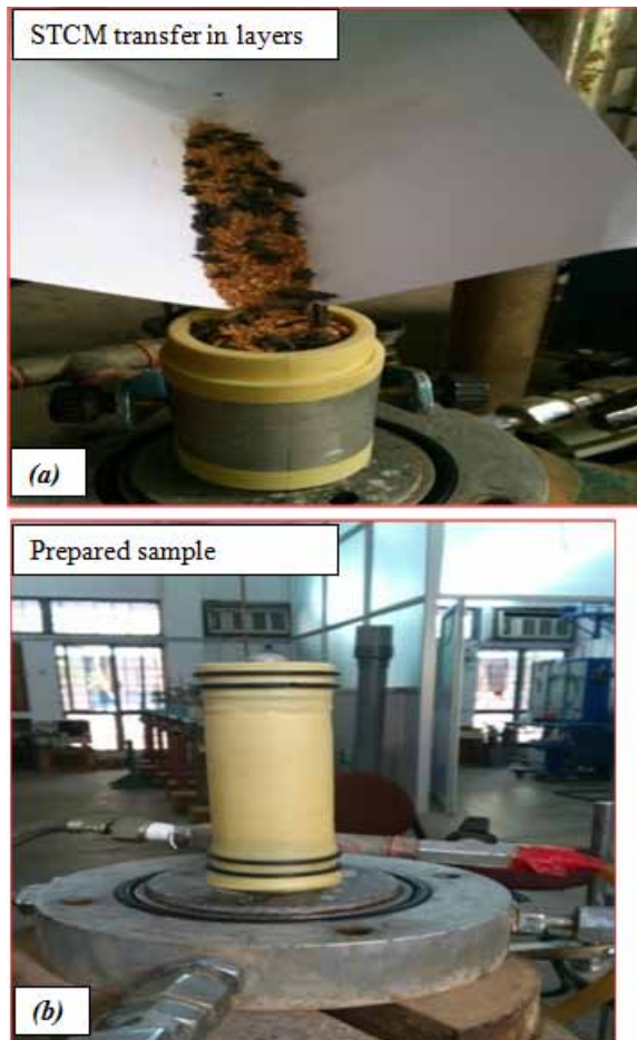
Figure 3. Typical photographs of STCM sample preparation for triaxial test
